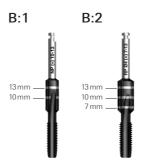
If the implant shoulder was planned below the bone crest, use the Guided Start Drill/ Counterbore to generate adequate access for the Guided Implant Mount. Select the Guided Start Drill/Counterbore matching the diameter of the implant.
