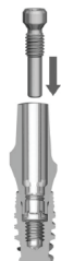
Figure C – Insertion of Abutment Retrieval Instrument into abutment (example with the Abutment Retrieval Tool Titanium CC)
