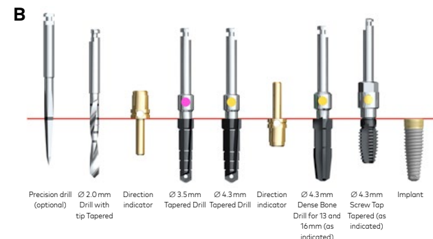
Figure B: Protocol steps and "Product Reference line" NobelReplace® CC TiUltra™, 13 mm long with regular platform
