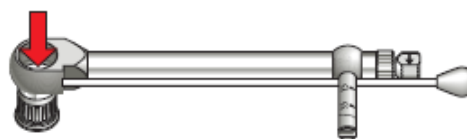
Figure D: Removal of Manual Torque Wrench Adapter
