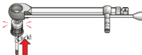
Figure F: Engagement of Adapter with Manual Torque Wrench
