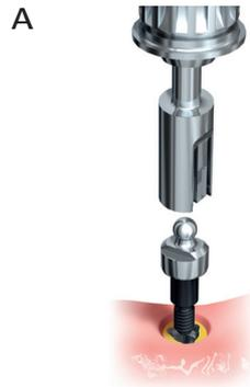
2. Tighten abutments to **15Ncm** using the Manual Torque Wrench Prosthetic and Screwdriver Machine Ball Abutment (B). If the Adapter for NobelReplace® WP to RP is used, push the ball abutment RP through the adapter into the implant and tighten to **15 Ncm** as described above (C).
