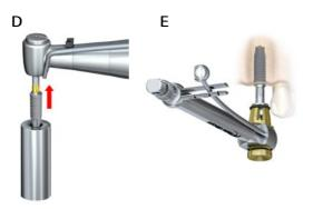
4. Place and tighten the implant using max. 45 Ncm insertion torque.
