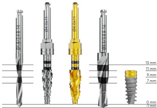
Figure D: Drill Depth Marking (Example for 4.0 x 11 mm Implant)
