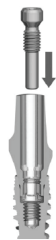
Figure E – Insertion of Abutment Retrieval Instrument into abutment (example with the Abutment Retrieval Tool Titanium CC)
