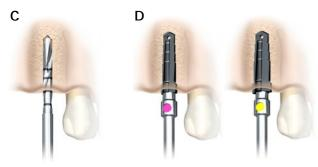
3. Open the implant package and pick up the implant from inner casing with implant driver (E). For conical connection implants it is recommended to applying light pressure on the implant driver and carefully turn the implant sleeve counter clockwise until implant driver is fully seated (E). The implants are ideally installed with low speed (maximum 25 rpm) using a drilling device or Manual Torque Wrench Surgical.
