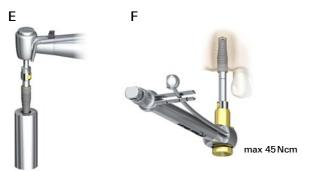
Place and tighten the implant using max 45 Ncm installation torque (F).
