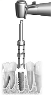
Figur F: Placering af Trephine Drill over implantat
