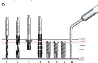
Drill reference lines for Twist Drill 7–15 mm (1), Twist Step Drill 7–15 mm (2), Counterbore (3), Screw Tap 7–13 mm (4), Brånemark System® Mk III Groovy (5), Brånemark System® Mk III TiUnite® (6), Brånemark System® Mk IV TiUnite® (7) implants 13 mm and Depth Probe 7–18 mm (8).
