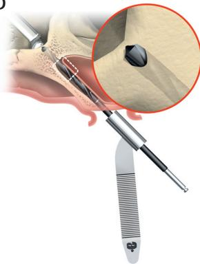
Depth measurement system: The parallel drills have a true depth measurement system. All drills and components are marked to prepare the site to the correct depth and obtain a secure and predictable position.
