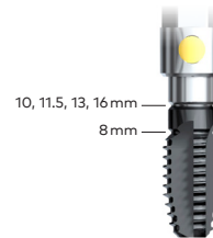
Figure G – Reference lines for implant length
